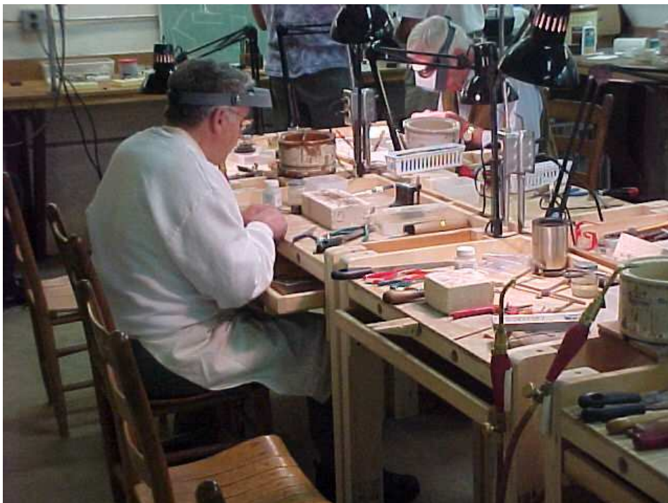
Silversmithing workshop at an SFMS Workshop. There are 12 individual workbenches with acetylene gas piped to torches into each position.
